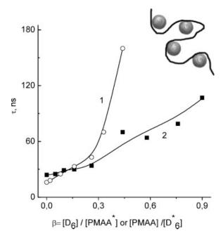
**Figure 1.** Dependence of  $\tau$  value on relation of interacting components  $\beta$  (in moles) in aqueous solution: PMAA\* and D<sub>6</sub> (1); PMAA and D<sub>6</sub>\* (2). Index \* means luminescently labeled component.
