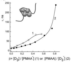
**Figure 2.** Dependence of  $\tau$  value on relation of interacting components β (in moles) in aqueous solution: PMAA\* and D<sub>3</sub>. (i); PMAA and D<sub>3</sub>\*(2). Index \* means luminescently labeled component.
